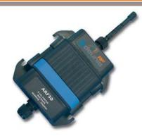
These systems enable one-way transmission of 8 digital states or 4 analog quantities over 4000m.
