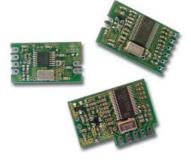
These transceivers enable an economic single-way **AM/FM digital link** over a range of **400m**. They are used as an asynchronous serial channel where the useful data rate ranges from **1.2 to 9.6kBps Manchester**. The transmission protocol remains up to the user.
