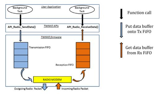
When the application calls the TWIMO\_API\_Radio\_SendData () function, a new element is put onto the transmission FIFO (FIFO size is 4 elements). Then the application does not have to deal with the transmission of the packet over the radio. The TWIMO firmware will proceed with the packet radio transmission as soon as it can.
